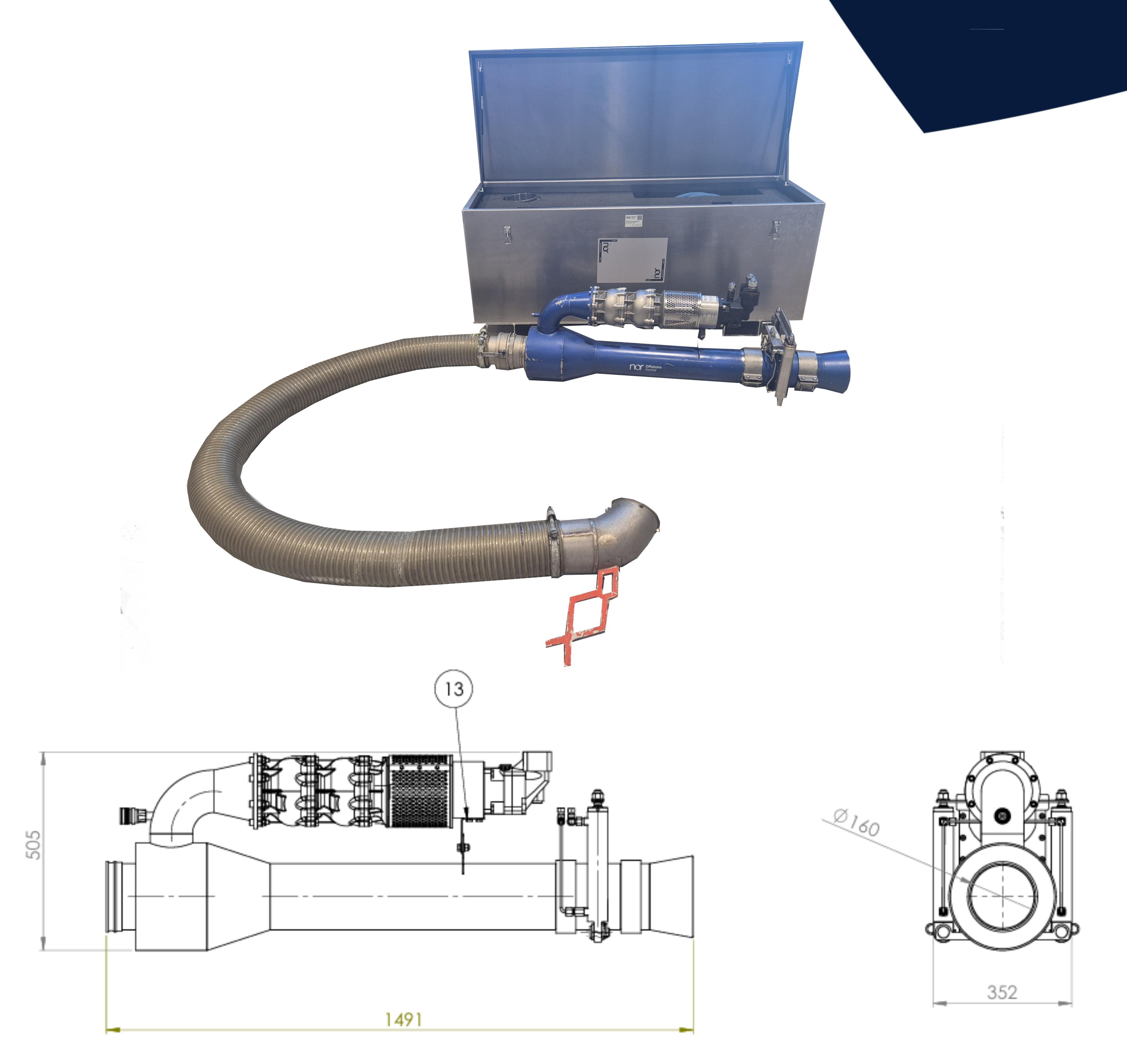
The NOR 6" ROV Dredge is a hydraulically powered, low-pressure seawater pump designed to work as an integrated opportunity to ROV subsea intervention. The efficient hydraulic energy can be utilized for salvage, excavating underwater pipelines system, dredging and similar underwater offshore intervention. The dredge system is also equipped with a hydraulically operated backflush mechanism designed to help with clogging issues.
