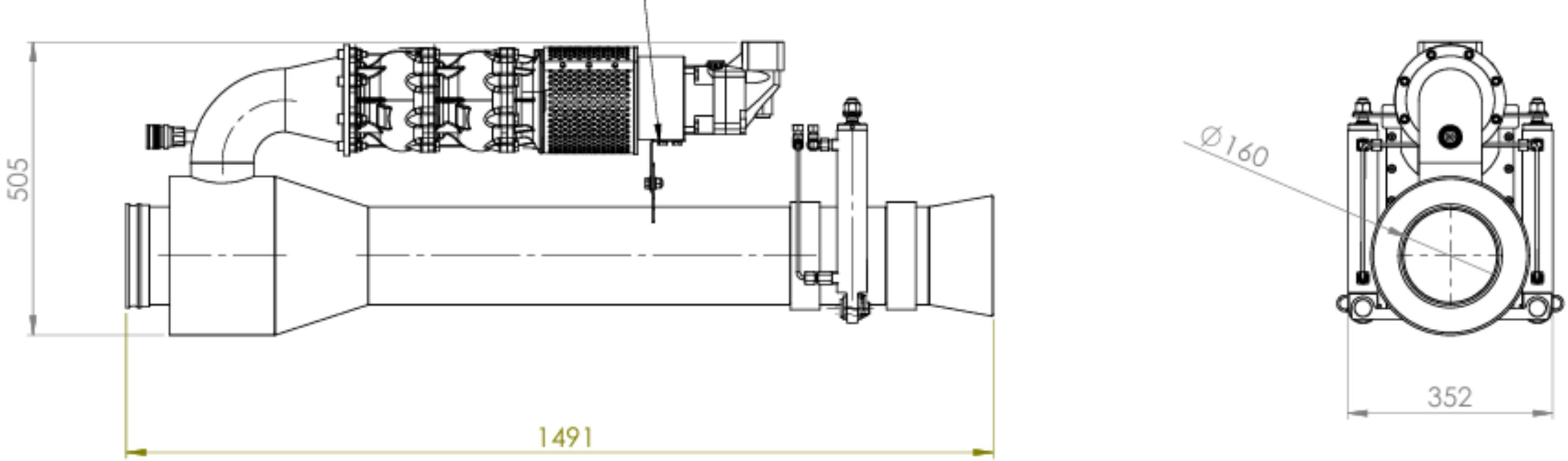
The NOR 6" ROV Dredge is a hydraulically powered, low-pressure seawater pump designed to work as an integrated opportunity to ROV subsea intervention. The efficient hydraulic energy can be utilized for salvage, excavating underwater pipelines system, dredging and similar underwater offshore intervention. The dredge system is also equipped with a hydraulically operated backflush mechanism designed to help with clogging issues.
