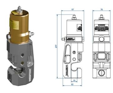
The WEBTOOL wire rope cutter WCO22D is designed for cutting medium diameter wire rope up to 22mm diameter in the most hostile environments, under the toughest of conditions. The wire rope cutter has an open sided design to allow easy positioning of the cutter along a rope length, which is particularly useful when cutting in confined spaces. It is supplied with hydraulic return ensuring full retraction of the blade.
