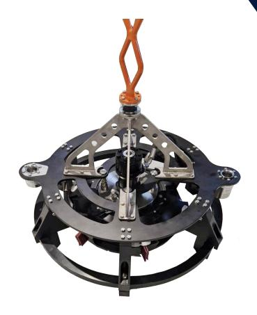
This manual is a user manual for the GNT Solutions P10825-GNT-R-MA-001 system. The Cleaning Tool is designed for cleaning XT-TOP 18-3/4" Wellhead seal surfaces. Designed for operations with and without tubing hanger installed. The Cleaning Tool consist of a main frame with a hydraulic driven cleaning disc. Handling of the Cleaning Tool by ROV Manipulator.
