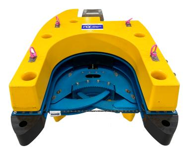
The NORSubsea Diamond Wire Saw is designed to be rugged and simple to use. It clamps onto pipes and cuts by operating the feed function on the wire. The saw can be operated by ROV with it's internal HPUin combination with hot stabs and Valve stabs, or Divers with the help of deck hose reel and HPU.
