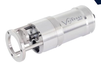
Aimed primarily at the underwater vehicle market, the uvSVX is a compact direct reading instrument that outputs a selectable, fixed data string at up to 60Hz of Sound Velocity, Temperature, Depth and optionally, Salinity and Density calculated with Valeport's proprietary DASH formula.
