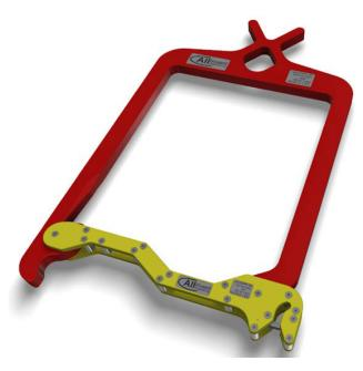
The subLOOPER® consists of 2 main parts hinged together. The biggest part is a fork with a ROV handle, and the small part can be hinged on both sides of the fork with a 2-way auto-lock hook at one end for the forerunner loop.
