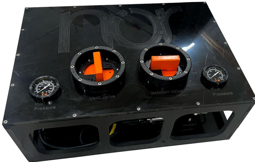
NOR PTU is used for pressure testing and can be set up in many various configurations, up to 10 000 PSI ( 700 bar). The PTU is small and easily integrated with subsea gauges, and has a built-in pressure sensor with logging capabilities.
