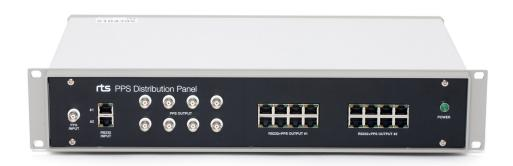
The RTS PPS distribution panel is the key solution for distributing GPS timing signals to survey spreads. It can be used to distribute one or two separate timing telegrams together with PPS pulse. The system consist of two RS232 splitters combined with three PPS pulse splitters. Selectable PPS pulse width, 500us, 1ms or directly from the GPS. Selectable PPS triggering, positive or negative edge. Typically used for time synchronisation of logging systems and multiple sensor synchronization.
