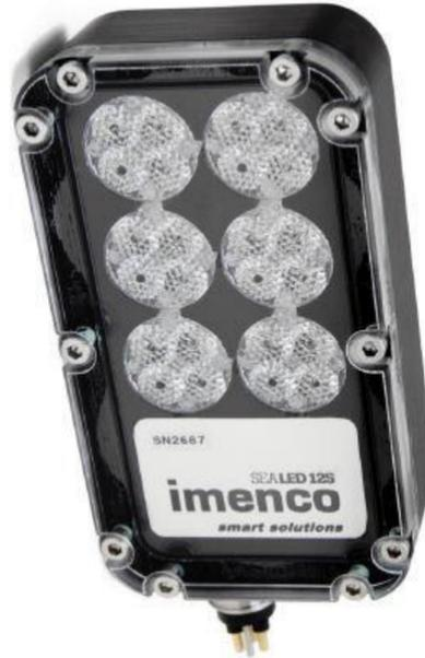
High output multipurpose SEA LED light panel for ROV / inspection points. Imenco SeaLED 125 is fitted with the latest high quality LED arrays which have a much longer lifespan than traditional Halogen / HID lights. SeaLED 125 can be delivered with different colour temperatures and lens angles. LED 125 light output is easily regulated from 0 - 100%.
