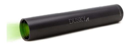
The Dusky Green Line Laser is a small size & low weight laser for Subsea measurements. The Dusky laser is a green line laser used when measurements are needed from video images. The green light ensures good visibility due to reduced absorption of green light in water.
