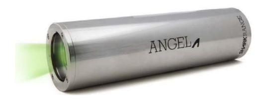
The Angel Laser is a powerful green line laser used when measurements are needed from video images. The green light ensures good visibility even at long distances due to reduced absorption of green light in water. By using two lasers in a fixed bracket, calibrated at set distance, accurate measurements from video images is possible
