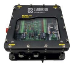
The CSS Torque Tool Control Valve Packs were designed to enable full control of hydraulic Torque Tool. Used with the CSS IVP and software we are able to offer repeatable control of Torque and Pressure. The Software provides control to the Board via RS232 / RS 485 which in turn can drive valves within the Valve Pack.
