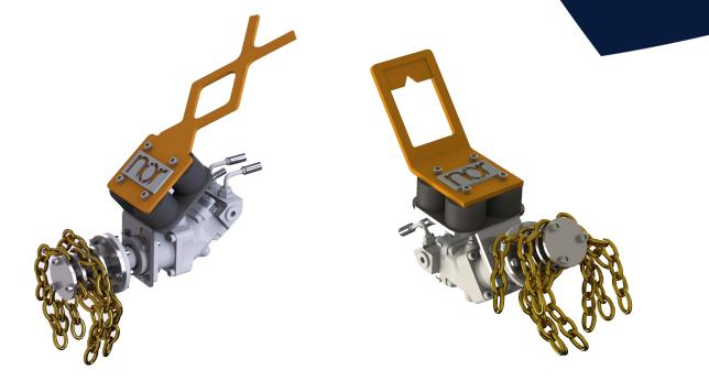
The NOR Chain Flain tool is designed for heavy duty cleaning work of marine growth, this is a powerful and robust tool which can be supplied with brass or steel chain links. Tool has anti shock mounting points which will help to not damage manipulators during operation.
