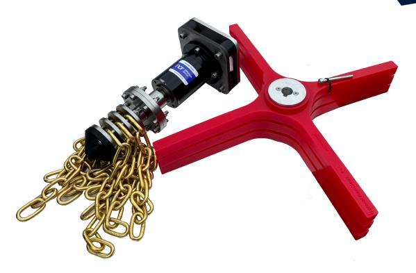
The NOR Chain Flail tool is designed for heavy duty cleaning work of marine growth, this is a powerful and robust tool which can be supplied with brass or steel chain links. Tool has anti shock mounting points which will help to not damage manipulators during operation.
