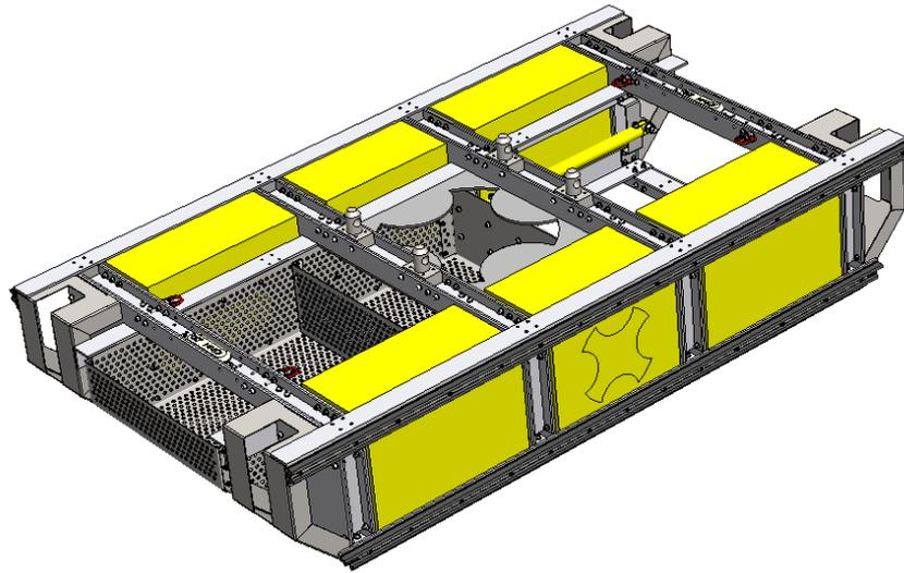
ROV Tool drawer skid can be fitted to many types of ROV's, and has space to install DWP, valve packs, IHPU's or any other applicable equipment which can be supplied by NOR. Here is also the possibility of adding more buoyancy to make it lighter in water. This is a very robust skid which can withstand heavy loads in harsh conditions.
