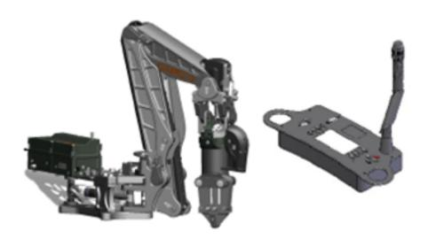
The Atlas Rate system may be installed on either the port or starboard side of the ROV and is available in two connector configurations. The Joint Sensor Kits are installed on to the exterior of the manipulator at each of the linear actuator joints (Azimuth, Shoulder, Elbow, Pitch and Yaw). A sensor cable is mounted on top of each kit.
