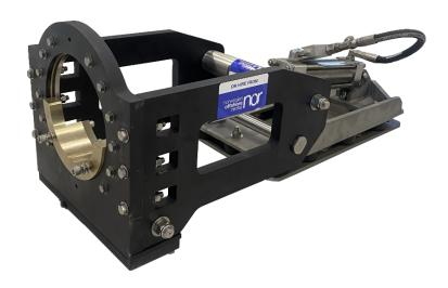
The FLOT was designed to be front mounted to an ROV for interface with various class 1-4 torque tools. The Docking cone was designed using a class 4 torque tool nose & latches. The FLOT has a total of 135° of pitch travel; 90° down from horizontal & 45° up from horizontal. FLOT has adapters for FORUM Torque Tool.
