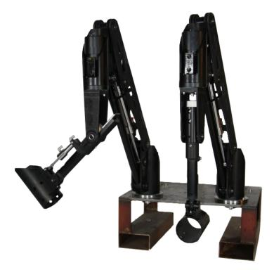
The Camera Boom is designed and built by KYSTDESIGN for use on survey ROVs. It is intended to be fitted with one customer supplied video camera and two Multi-SeaLite lamps. It has four hydraulic functions - boom rotate, elevate, pan and tilt. The lower section will release and pivot on impact. The pivoting section is held into position by two strong magnets.
