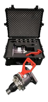
ISO/17D Class 4 to Petrobras Adaptor is an interface extension, designed to allow Petrobras valve interfaces to be actuated using a class 4 torque tool. It is a purely mechanical tool designed to be used with an ISO 17D Class 4 Torque tool, utilising its latching capability to secure the adaptor.
