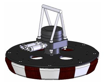
The Motorized Wellhead Cleaning Tool is designed to clean the seal surface of wellheads that use AX or VX gaskets. The ROV powers the tool and holds it in position to remove debris. Flow regulator valves limit the rotation speed while still allowing high torque.
