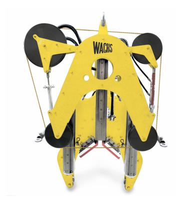
The Wachs Subsea Diamond Wire Saws are designed for underwater cutting of horizontal or vertical pipe, casings and structure, with five models that cut from 4in to 84in O.D. (DN100-DN2100). Running on hydraulic power, the wire saw is controlled remotely using the Wachs Topside Control Panel (TCP), Wachs HPU with integrated TCP or by ROV control operable via zero leak hot stabs.
