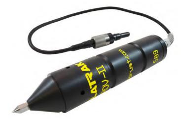
General Polatrak ROV II is a self-contained ROV-mountable or diver-operated cathodic protection meter/probe. The unit allows the operator to probe a submersed structure to determine its electrochemical potential. Features twin reference electrodes and dual ultrabright digital readouts (when using Polatrak's Deep C Meter).
