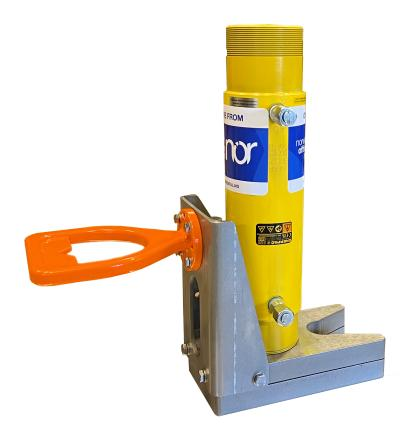
The Override 3te Subsea Jack is a bolted construction built with a double-acting cylinder, and stainless steel components. It is standard and common to use the ROV HPU to operate the tool/cylinder. The maximum pressure for this tool (100 bar) corresponds to approximately (31.7kN) 3200 kg separating force.
