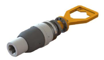
The Manual Torque Tool or Torque Limiter is designed to allow the ROV manipulator operation of Petrobas Specification rotary torque interfaces. The tool limits the torque that can be transmitted from the ROV manipulator to the valve stem during an ROV intervention operation, mitigating against the possibility of over-torqueing and damaging the valve or valve stem. The tool is fitted with an integral, adjustable torque limiting clutch which can be pre-set to any torque from 20 – 200Nm.
