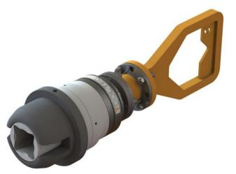
The Manual Torque Tool or Torque Limiter is designed to allow the ROV manipulator operation of ISO 13628-2 / 17H Specification rotary torque interfaces. The tool limits the torque that can be transmitted from the ROV manipulator to the valve stem during an ROV intervention operation, mitigating against the possibility of over-torqueing and damaging the valve or valve stem. The tool is fitted with an integral, adjustable torque limiting clutch which can be pre-set to any torque from 20 – 200Nm.
