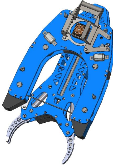
The NOR Subsea **Diamond Wire Saw** is designed to be rugged and simple to use. It clamps onto pipes and cuts by operating the feed function on the wire. The saw can be operated by ROV with its internal HPU in combination with hot stabs and Valve stabs, or Divers with the help of deck hose reel and HPU.
