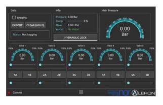
5-Station Valve pack is a very versatile system which can be integrated to almost any skid or backpack. It has a touchscreen software which is capable of operating all the valves proportionally, with accurate pressure and flow control. The software also is capable of logging and exporting data, which will give you very good control over monitoring pressure and flow on external tooling. Valve pack is set up with 3 external sensors to monitor compensator, pressure sensor and flow rate sensor.
