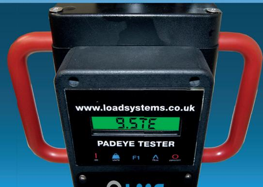
Lightweight, portable tool for testing pad eyes, lifting lugs, and eye bolts. It can be used upright, inverted, or in a horizontal plane. Models are available up to 60 ton proof test capability. Equipped with an adjustable clevis height and Digital Mounted Display.
