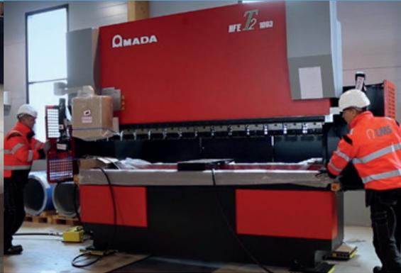
Air skates are robust, low profile, high capacity load-moving modules used in sets of four or six to enable large or heavy objects to be moved with ease.
