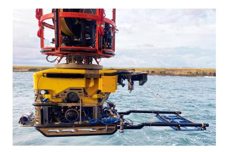
Kystdesign pipetracker hydraulic frame can be mounted on the back or front on the subsea vehicle, can be used on various ROV's, Trenchers, Excavation machines etc. Mounting brackets can be supplied with, which also have the possibility of integrating Kystdesign camera booms.
