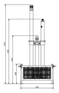
Guidepost/extension basket is used for lifting guidepost safely to seabed and installing them on subsea assets. Center Pole basket can be re-modified to multipurpose basket with or without hatches.
