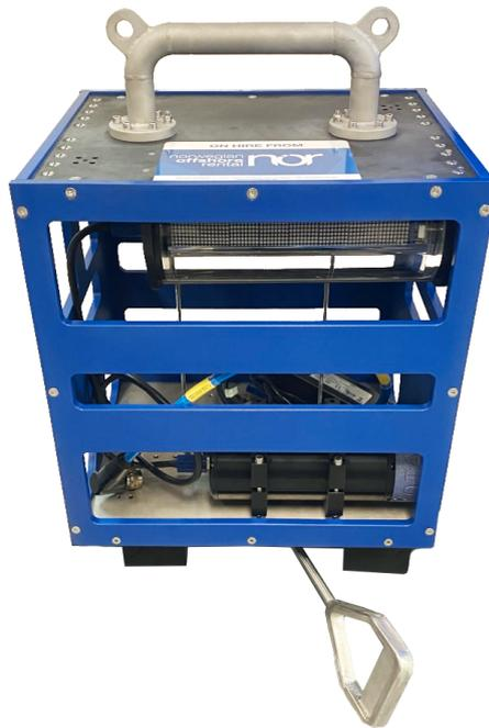
Gyro frame is used for subsea structure positioning or as a standard inclinometer. Heading, roll and pitch read out on the subsea display with different possibilities of accurate positioning. Can also be used with MET stab, which receptacle can be pre-installed on structure.
