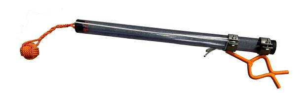
When the NOR dye stick injection tool is combined with our HPW Jetter you are able to inject dye sticks into well heads, hubs, and other structures subsea. It has a cap in front to prevent dye sticks from falling out. The cap can be removed either by ROV or the water pressure. Cap is secured with a bungee cord.
