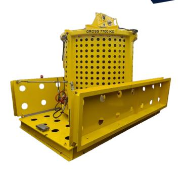
The 5450 litre Subsea Reservoir is a pressure compensated collapsible reservoir with protective cage and mudmat for safe deployment and recovery. It is utilized in the deployment, injection or recovery of fluids to and from equipment residing on the seafloor. Other tooling can be integrated as DWP, IHPU or HPW Pump.
