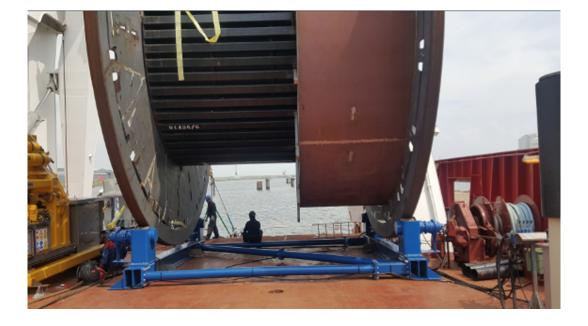
The under-roller spread is delivered as a "turn-key" solution, including user manual, el- and hydraulic diagrams, flow sheet aswell as spare hoses and connections.
