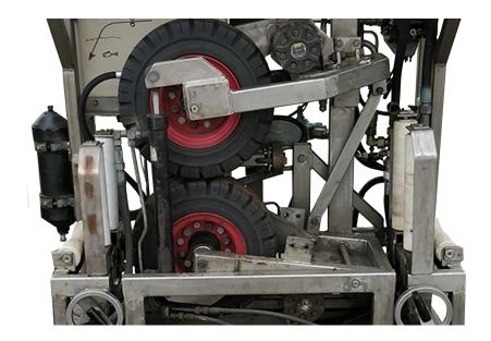
Easy to use, 1-wheel pair tensioner with a small footprint, perfect for HV-cables.
