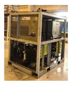
Hydraulic Power Unit in Certified frame with PVG valves. Easy to use and robust design, great for deck testing.
