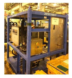
Hydraulic Power Unit in Certified frame with PVG valves. Easy to use and robust design, great for deck testing.
