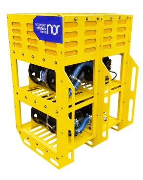
The High Flow DWP is a compact isolated hydraulic system, which is easily integrated into a ROV System. It is a very versatile system which can be integrated with various options of set up and features.
