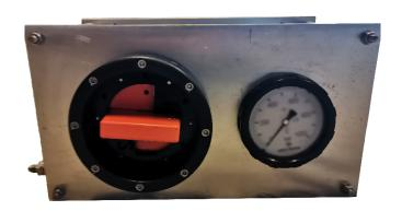
The Back Seal Test Panel consists of a ROV operated isolation valve, pressure gauge and mini booster. This will allow you to log and monitor the pressure on a typical back seal test. There is also an option for having this with a ISD4000 pressure sensor, which will allow you to log and have pressure feedback through software. Panel can be mounted on the manipulators, belly basket or any other place where the Schilling T4 has access to it.
