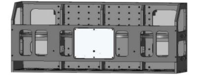
NOR ROV intervention backpack is a lightweight rack which can hold 4x 16ltr compensators. This can be fitted to the back of the ROV and will enable the ROV to hold fluids up to 64ltr. This can be used for fluid injection or to operate subsea tooling which requires a large amount of hydraulic oil. Can be connected to NOR IHPU, DWP etc.
