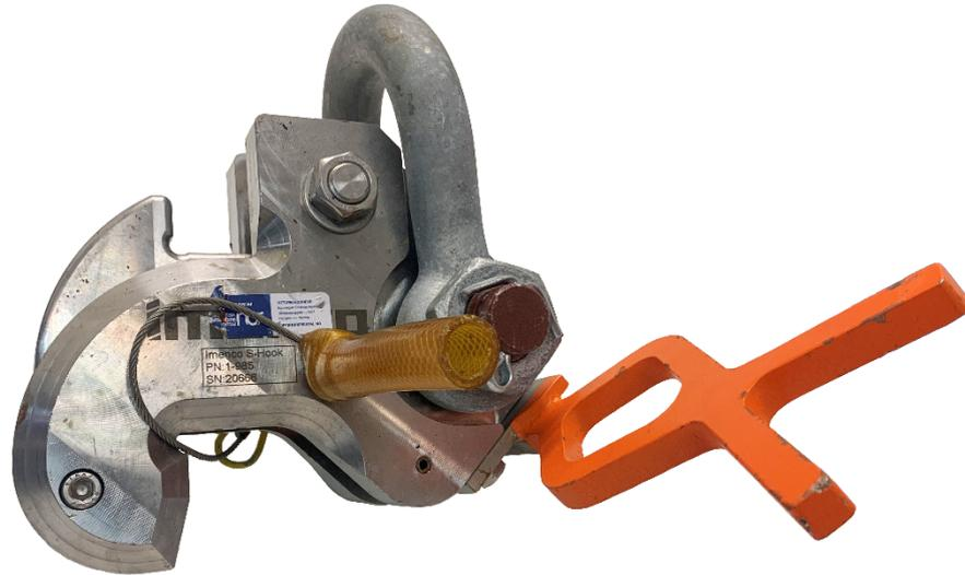
The Imenco S-Hook Lifting Anchor is developed with a purpose to achieve a safe handling when steel structures e.g. riser pipes are being removed during demolition and decommissioning of offshore structures. The Imenco S-Hook Lifting Anchor is designed for loads in parallel to normal direction relative to the riser. The anchor is furthermore equipped with a self-locking latch dog that will automatically activate when the anchor is correctly mounted into a pre-drilled anchoring hole.
