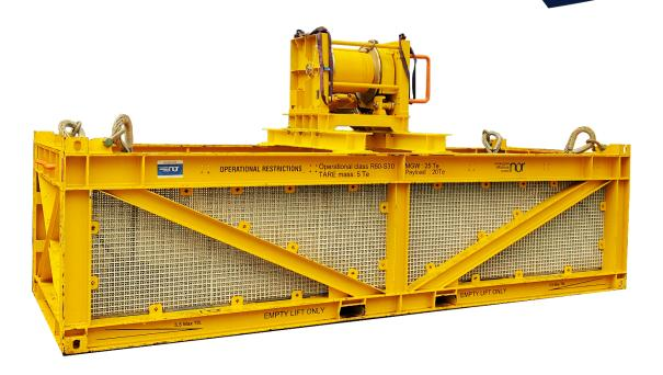
The Subsea Winch 5Te is intended for offshore subsea pulling operations. It is designed to withstand rough operations in any offshore environment. With a full 360° rotating drum this winch allows for a 5Te line pull on a horizontal plane. The winch is operated locally and powered hydraulically from an external HPU, which is supplied by ROV via a quick-acting coupling live Hot Stab.
