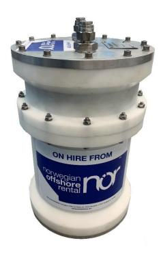
The ROV and Subsea Hydraulic Compensator ensures system overpressure at all times. The Imenco Hydraulic Compensator is a spring activated diaphragm compensator, made from white POM with aluminium lids on the top and bottom. The spring and all bolts and nuts are stainless steel.
