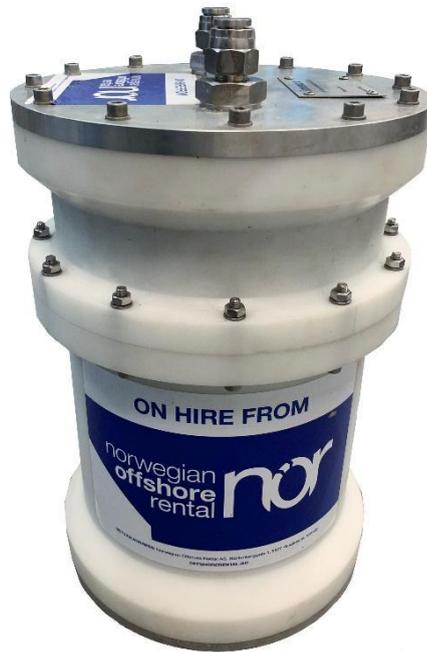
The ROV and Subsea Hydraulic Compensator ensures system overpressure at all times. This is the Imenco Hydraulic Compensator is a spring activated diaphragm compensator, made from white POM with aluminium lids on the top and bottom. The spring and all bolts and nuts are stainless steel.
