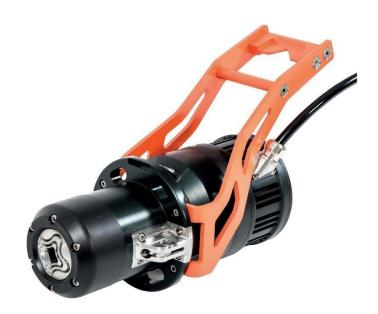
The Universal Electrical Torque Tool is designed to improve operational efficiency with the highest level of performance. The eTorque Tool provides precise torque and turn feedback and control. It is able to operate all rotational valves continuously when submersed, without the need for any change of motor size, gears steps or valve interfaces, and thereby saves valuable rig/vessel time.
