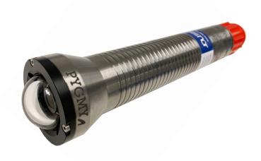
The OE17-101 Pygmy, is a compact and versatile HDIP colour subsea tooling camera offering excellent video quality with up to 1920 x 1080-pixel resolution at 30 fps. The camera utilises a 1/2.8" CMOS sensor and supports both H.264 and MJPEG video compression standards for transmission over a 10/100 Base TX Ethernet network connection.
