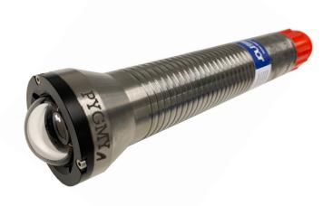
The OE17-101 Pygmy, is a compact and versatile HDIP colour subsea tooling camera offering excellent video quality with up to 1920 x 1080-pixel resolution at 30 fps. The camera utilises a 1/2.8" CMOS sensor and supports both H.264 and MJPEG video compression standards for transmission over a 10/100 Base TX Ethernet network connection.
