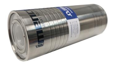
The Imenco Whitetip Shark<sub>HD</sub> Colour Zoom Camera incorporates a 4Mpx - 1/3" CMOS sensor and features a 10x optical zoom lens. With built-in LED lights and ultra-compact and lightweight Titanium body rated to 4.000msw, it is an ideal camera for inspection of restricted spaces and for use in tooling.
